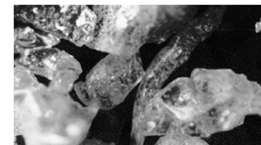
Slag is changed to glassy sand like substance known as granulated blast furnace slag - GBFS
