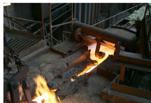
Slag Diverted to Granulator High pressure water 6 - 10 tons water/ton slag
