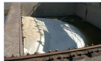
Slag is changed to glassy sand like substance known as granulated blast furnace slag - GBFS
